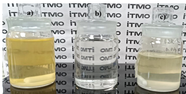
Fig. 2. Changes in the color and consistency of the sol depending on the synthesis temperature: (a) 201–220 °C, (b) 195–200 °C, (c) below 195 °C.
